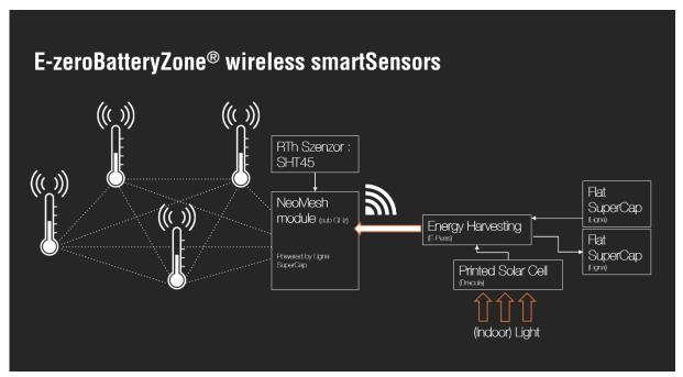
The node architecture is very similar whether using various low-power analog or digital sensors. It consists of a sensor—connected either to an ADC pin or an I2C channel of the NeoCortec communication module's internal ARM Cortex M0+ microcontroller—and an energy harvesting unit. The latter primarily comprises a photovoltaic cell capable of operating under low indoor illumination, the energy harvesting IC, and specialized supercapacitor cells.
