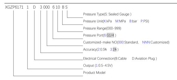
Note: The default length of Aviation-Plug wire: 1 meter; contact CFSensor for any customized wire length,
