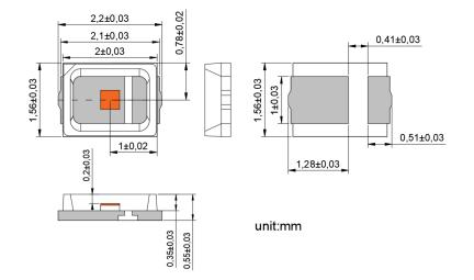
VD-0940V-800M-1A-2B0 with Substrate 1=AIN and Package A=2016 (unit: mm)
