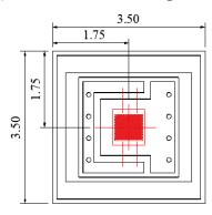
VD-0940V-400W-5H-3B0 (Substrate FeNi Alloy, Package TO56)
