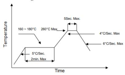
**Note:** Reflow soldering can be operated only one time. During the temperature ramp-up, no forces may be exerted on the diode which could deform or damage them. After soldering completed, please also do not process until the product temperature ramp down to room temperature.
