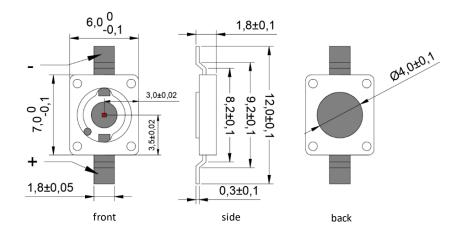
VD-0940I-400M-1A-2A0 with Substrate 1=AIN and Package A=2016 (unit: mm)
