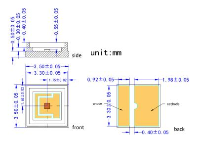
VD-0940I-400M-3E-2A0 with Substrate 3=<u>Cu/Aq</u> and Package E=<u>7060</u> (unit: mm)
