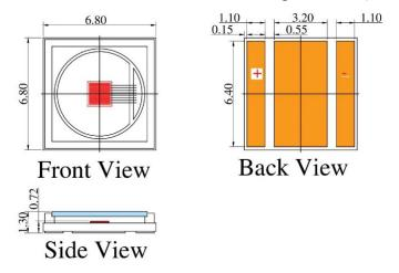
VD-0940I-006W-6K-2B0 with Substrate 6=Cu and Package K=T-mount (unit: mm)
