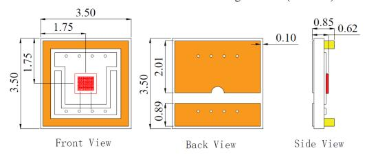
VD-0940I-006W-1D-2B0 with Substrate 1=AIN and Package D=5050 (unit: mm)
