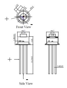
VD-0940C-010M-3W-2A0 with Substrate 3=<u>Cu/Ag</u> and Package Plastic Dip W=<u>0428</u> (unit: mm) (Remarks: Operating only in pulsed mode)
