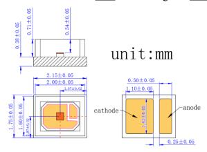
VD-0940C-010M-3A-2A0 with Substrate 3=<u>CuAg</u> and Package A=<u>2016</u> (unit: mm)
