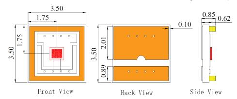
VD-0850I-130M-3A-2A0 with Substrate 3=<u>Cu/Ag</u> and Package A=<u>2016</u> (unit: mm)
