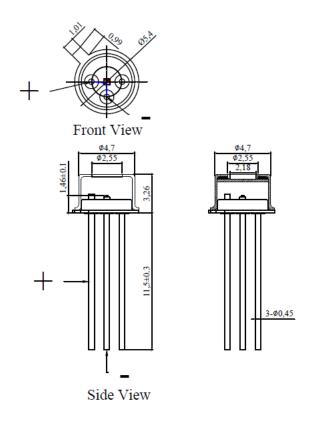
VD-0850C-010M-3W-0A0 with Substrate 3=<u>CuAg</u> and Package Plastic Dip W=<u>0428</u> (unit: mm)
