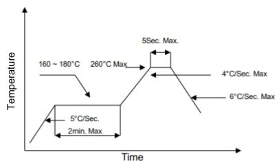
Note: Reflow soldering can be operated only one time. During the temperature ramp-up, no forces may be exerted on the VD which could deform or damage them. After soldering completed, please also do not process until the product temperature ramp down to room temperature.
