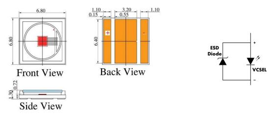
VD-0808I-007W-6K-2A0 with Substrate  $6=\underline{Cu}$ , Package  $K=\underline{T\text{-mount}}$  (unit: mm), and ESD protection diode
