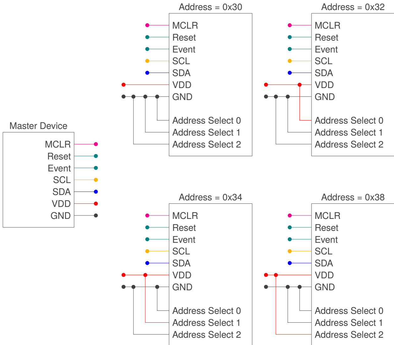
Figure 5.1: Multiple Devices with I 2 C Interface
