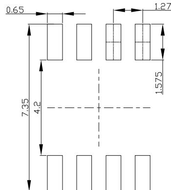
For PCB assemblies that cannot support a slotted design, the above stretched footprint may be used
