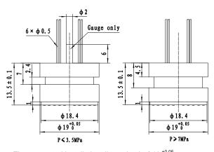
The suggested installation dimension is  $\Phi 19\,^{+0.05}_{+0.02}\,\text{mm}$
