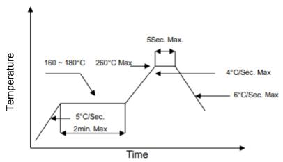
Note: Reflow soldering can be operated only one time. During the temperature ramp-up, no forces may
