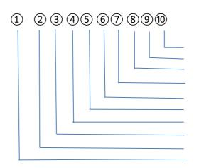
Annex, option 0 Product version, A Accessories, 0= standard Package type, 3528 Substrate, 4= P/Cu Power units, M =milliwatts Power, 200
