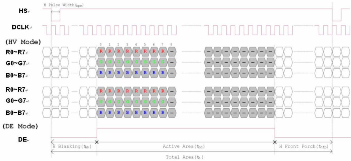
Figure 1.1 Horizontal input timing diagram
