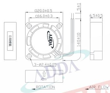
LEAD WIRES: UL 1571, AWG28, L = 140 +/- 10 mm Red = positive; Black = negative.
