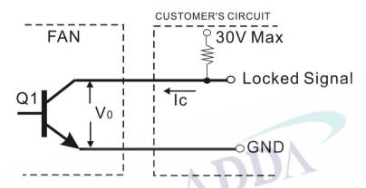
\*Transistor Q1 at "ON" position
