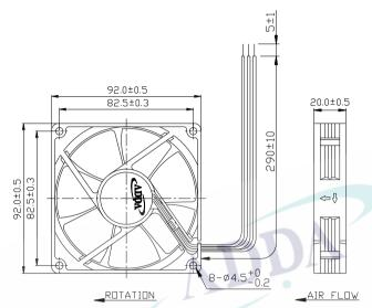
LEAD WIRES: UL 1007, AWG24, L = 290 +/- 10 mm Red = positive; Black = negative.
