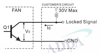
\*Transistor Q1 at "ON" position
