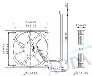
LEAD WIRES: UL 1007, AWG24, L = 290±10 mm Red = positive; Black = negative. Blue =FG
