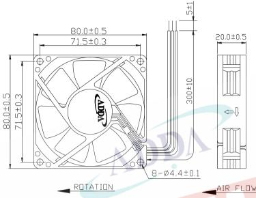
LEAD WIRES: UL 1007, AWG24, L = 300± 10 mm
