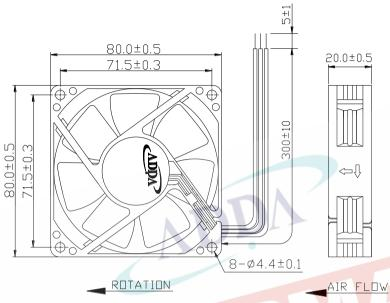
LEAD WIRES: UL 1007, AWG24, L = 300±10 mm Red = positive; Black = negative. White = FG
