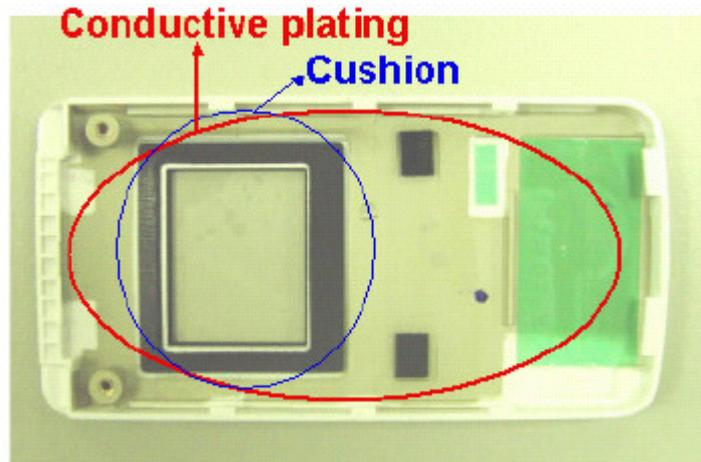
It is recommended that a plating conductive layer be used in the housing for EMI/EMC protection. And, the enough space should be reserved for the IC placement if the IC thickness is thicker than the TAB film when customer design the PCB.
