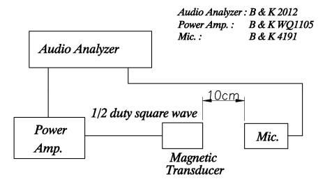
7. Standard driving circuit for transducer
