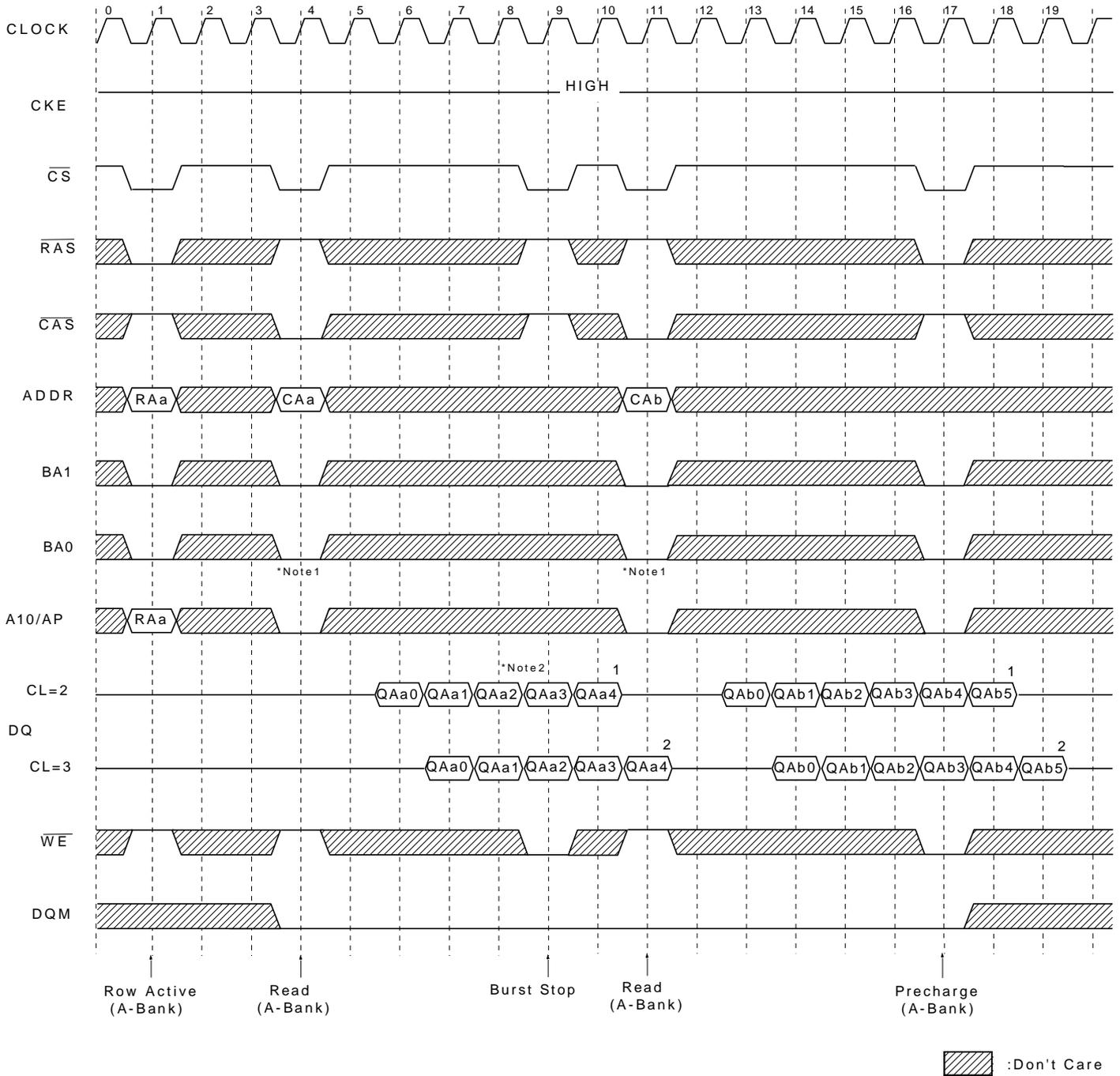
\*Note: 1. About the valid DQs after burst stop, it is same as the case of  $\overline{\text{RAS}}$  interrupt. Both cases are illustrated above timing diagram. See the label 1, 2 on them. But at burst write, Burst stop and  $\overline{\text{RAS}}$  interrupt should be compared carefully. Refer the timing diagram of "Full page write burst stop cycles".
