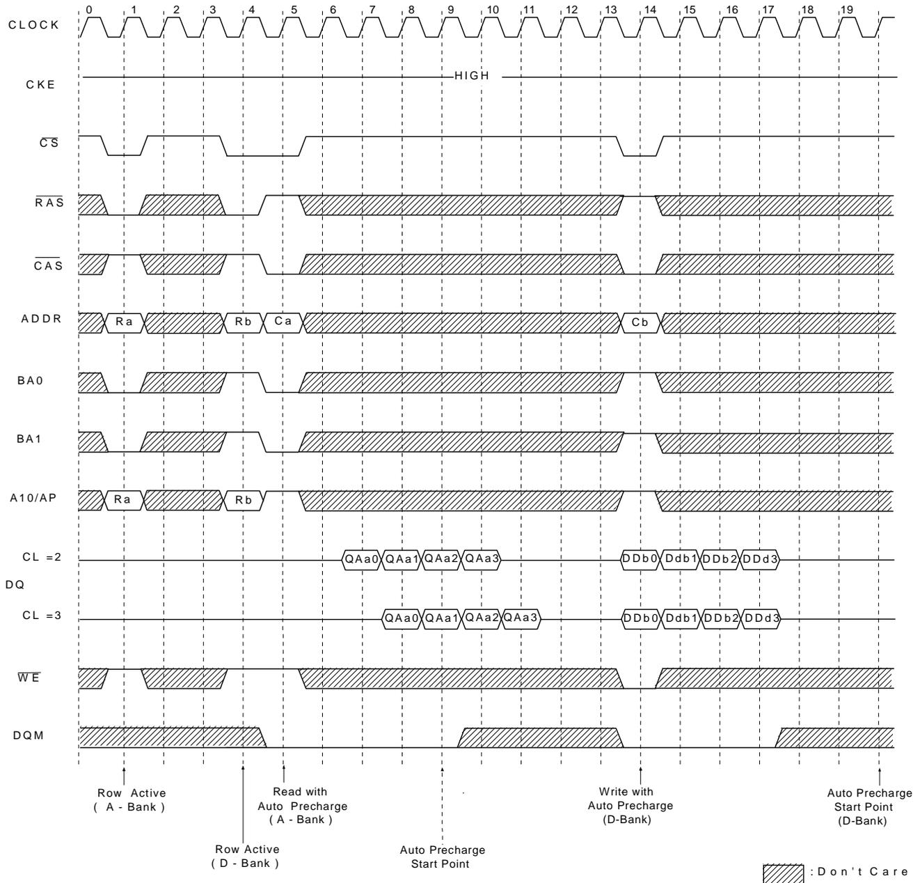
\*Note: 1. t<sub>CDL</sub> should be controlled to meet minimum t<sub>RAS</sub> before internal precharge start.
