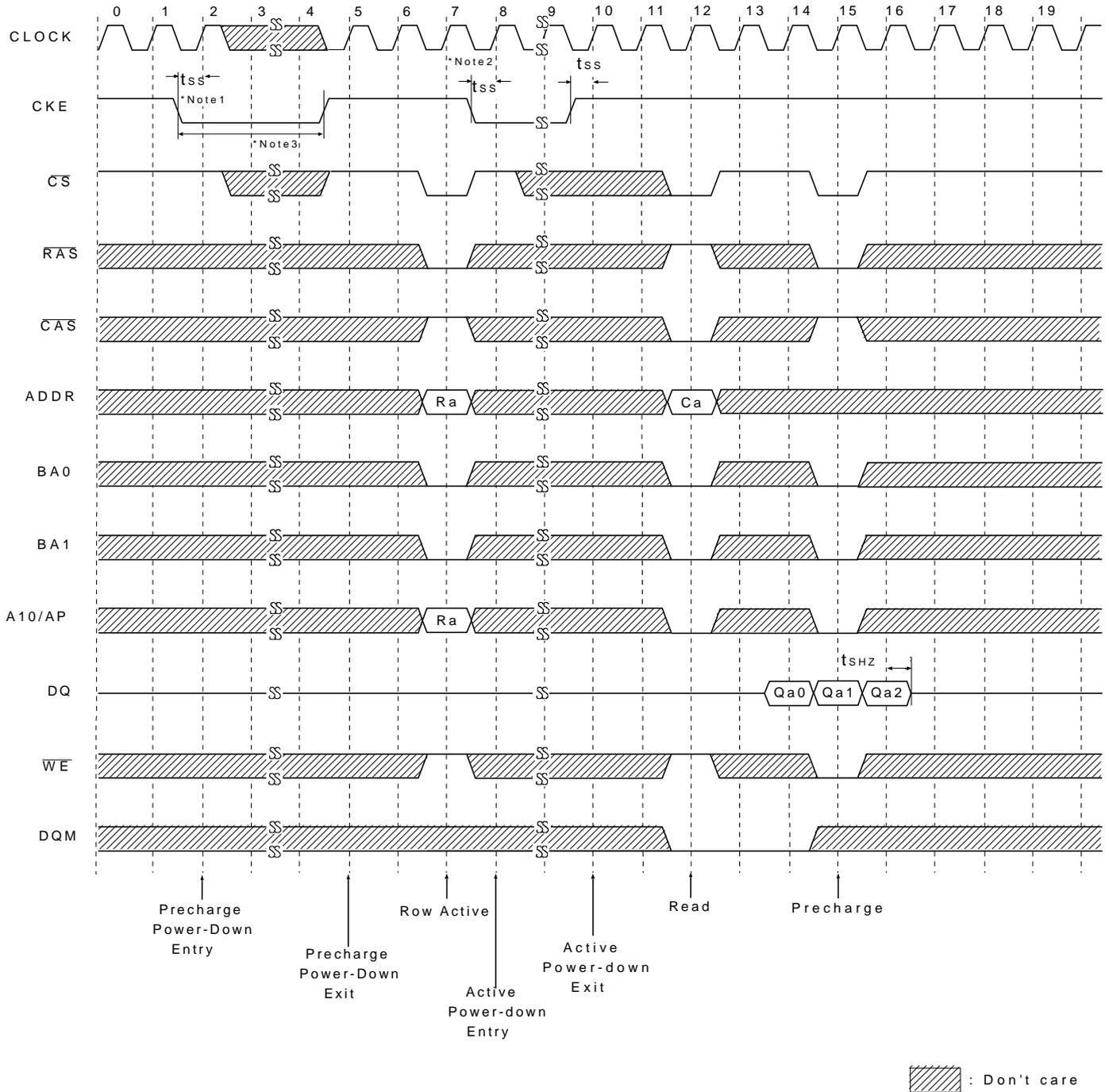
\*Note: 1. All banks should be in idle state prior to entering precharge power down mode.
