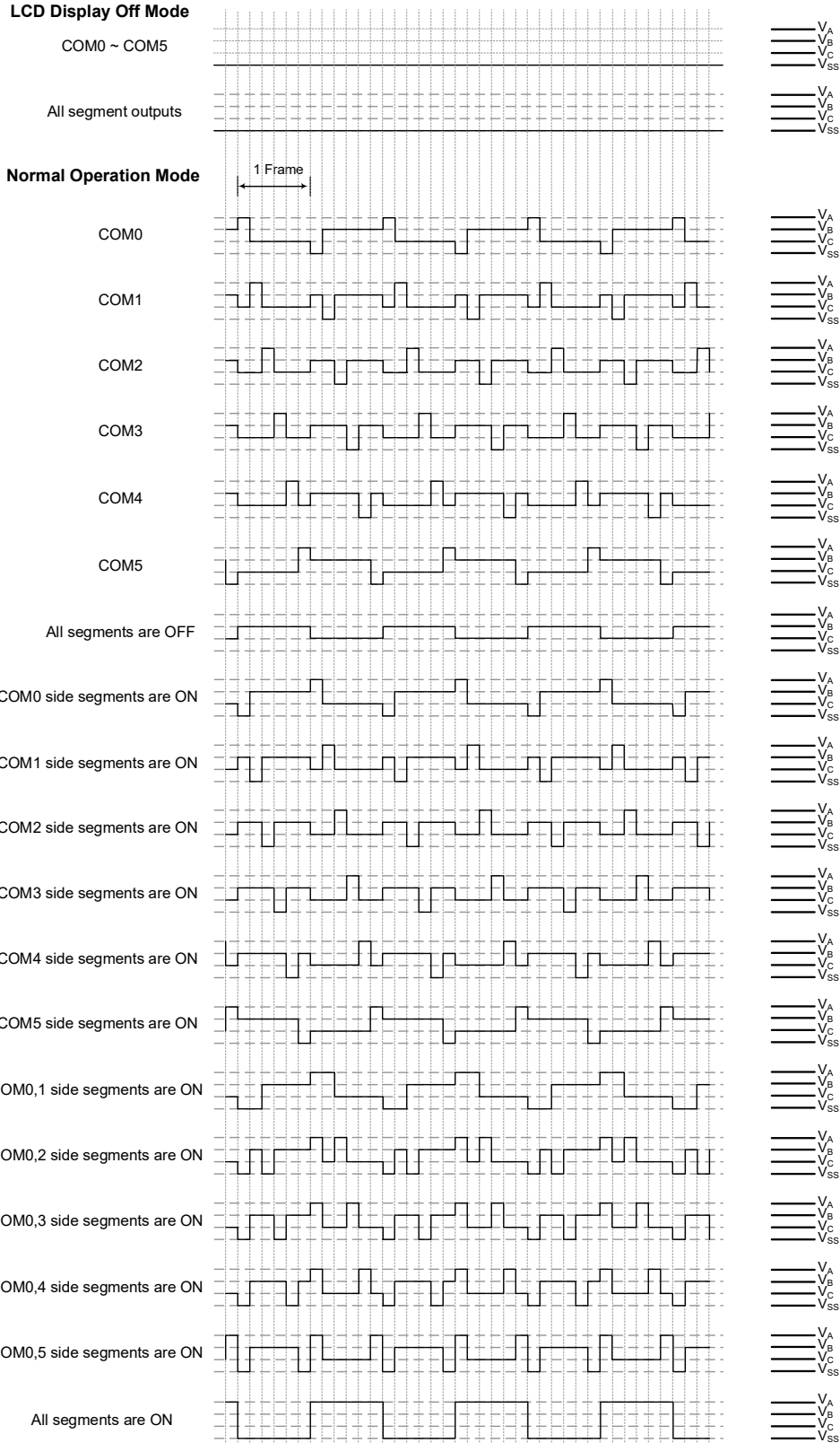
LCD Driver Output – Type B, 1/6 Duty, 1/3 Bias
