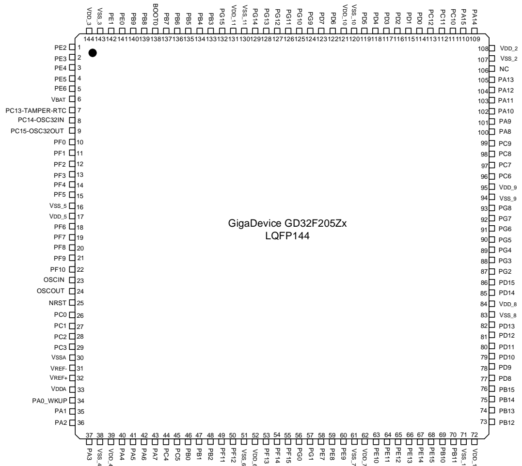
Figure 2-2. GD32F205Zx LQFP144 pinouts
