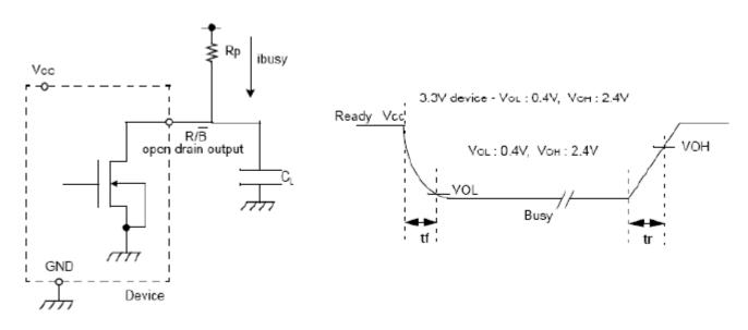
R<sub>P</sub> vs t<sub>RHOH</sub> vs C<sub>L</sub>
